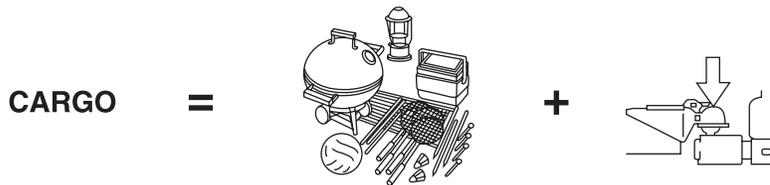
**Cargo Weight** – includes all weight added to the Base Curb Weight, including cargo and optional equipment. When towing, trailer tongue load or king pin weight is also part of cargo weight.
