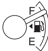
The arrow near the fuel pump icon indicates which side of the vehicle the fuel filler door is located.
