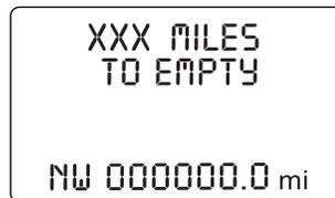
The DTE function will display LOW FUEL LEVEL and sound a tone for one second when you have approximately 50 miles (80 km) to empty. If you RESET this warning message, this display and tone will return within 10 minutes or 10 miles (16 km).
