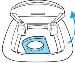
5. Clip the tether strap to the anchor as shown.
