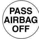
**Note:** The indicator lamp will illuminate for a short period of time when the ignition is turned to the ON position to confirm it is functional.
