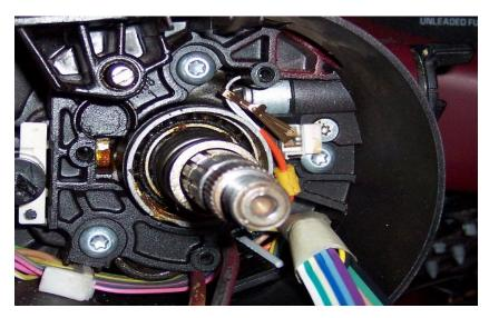
This is what the inside of the steering column looks like torn apart down to the ignition lock cylinder. Just to the right of the steering shaft, you can see the orange "conduit" with the 2 white wires running out of it into the lock cylinder. These wires typically break off inside the column, rendering the reader useless. The purpose of this document is to save the hassle of tearing the column apart, and get the car up and running for the least amount of cost.
