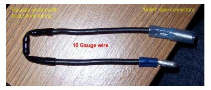
Notice in the above "resistor pack" I lucked out and only needed 1 resistor to match the pellet's resistance. You may not be so lucky...
